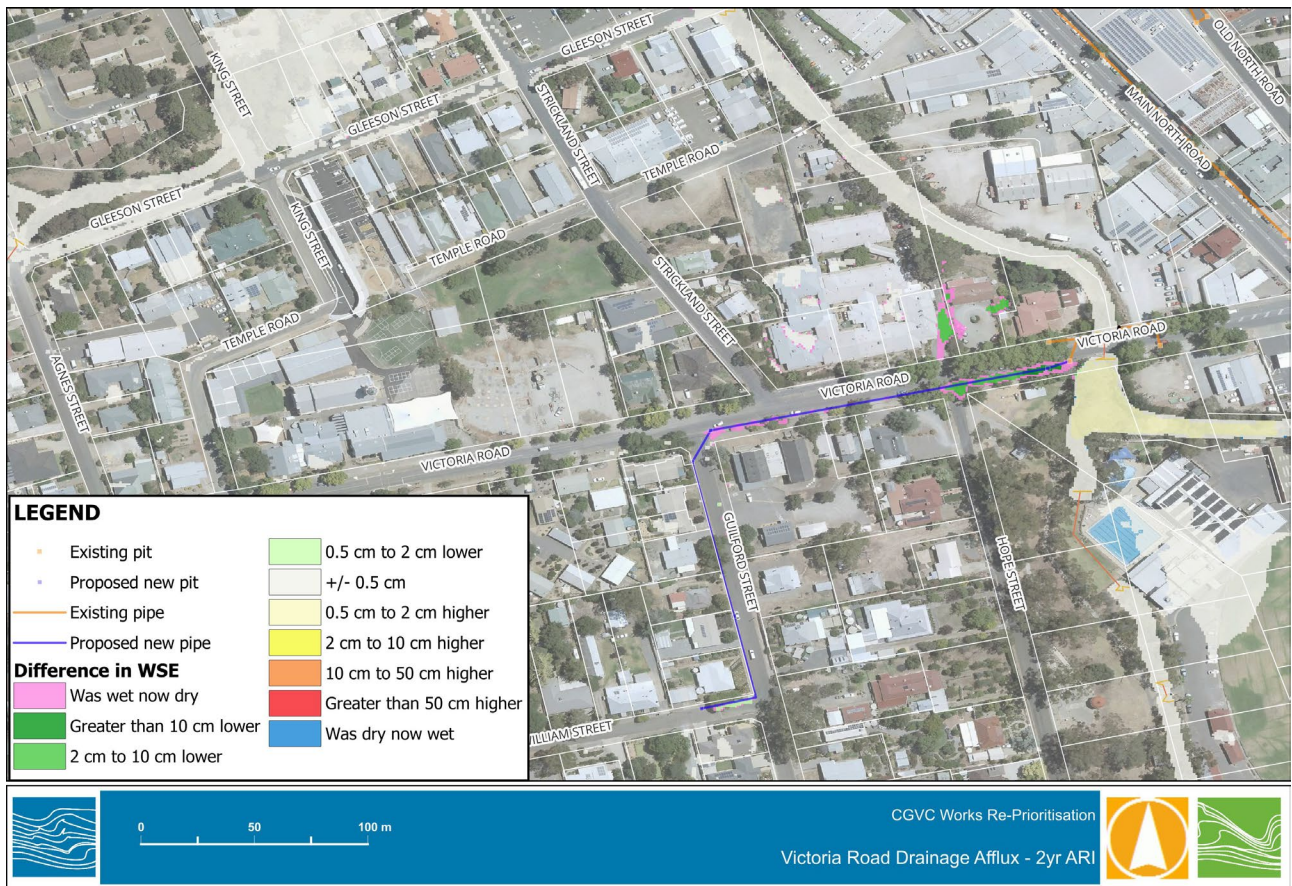
Figure 5-9 Difference in water level between proposed Victoria Rd drainage works and existing conditions (2-year ARI local rainfall event)
