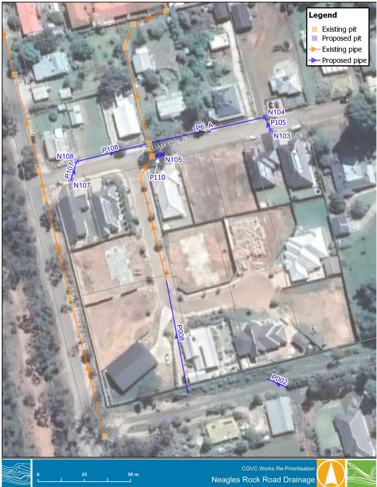
Figure 4-3 Neagles Rock Road drainage upgrade schematisation
