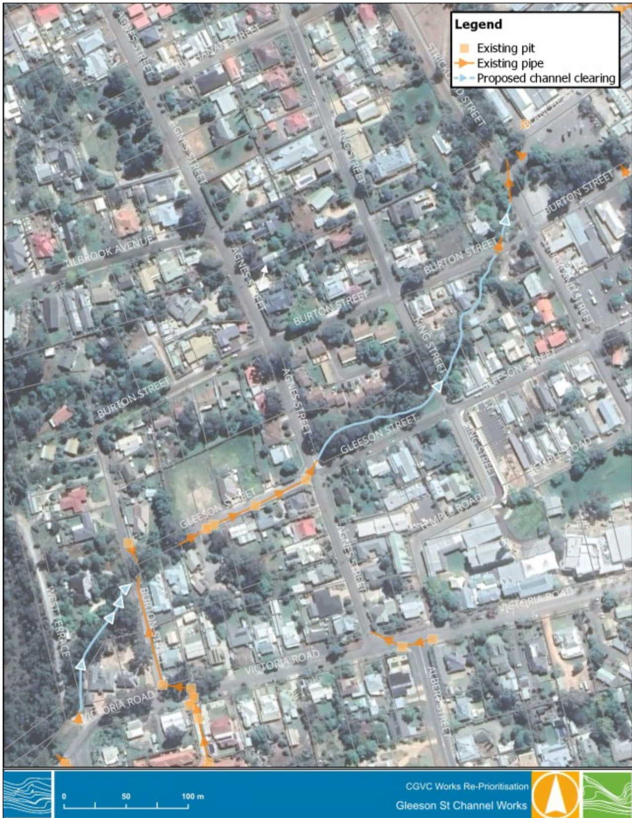
Figure 4-10 Extent of Gleeson trunk main channel maintenance/clearing
