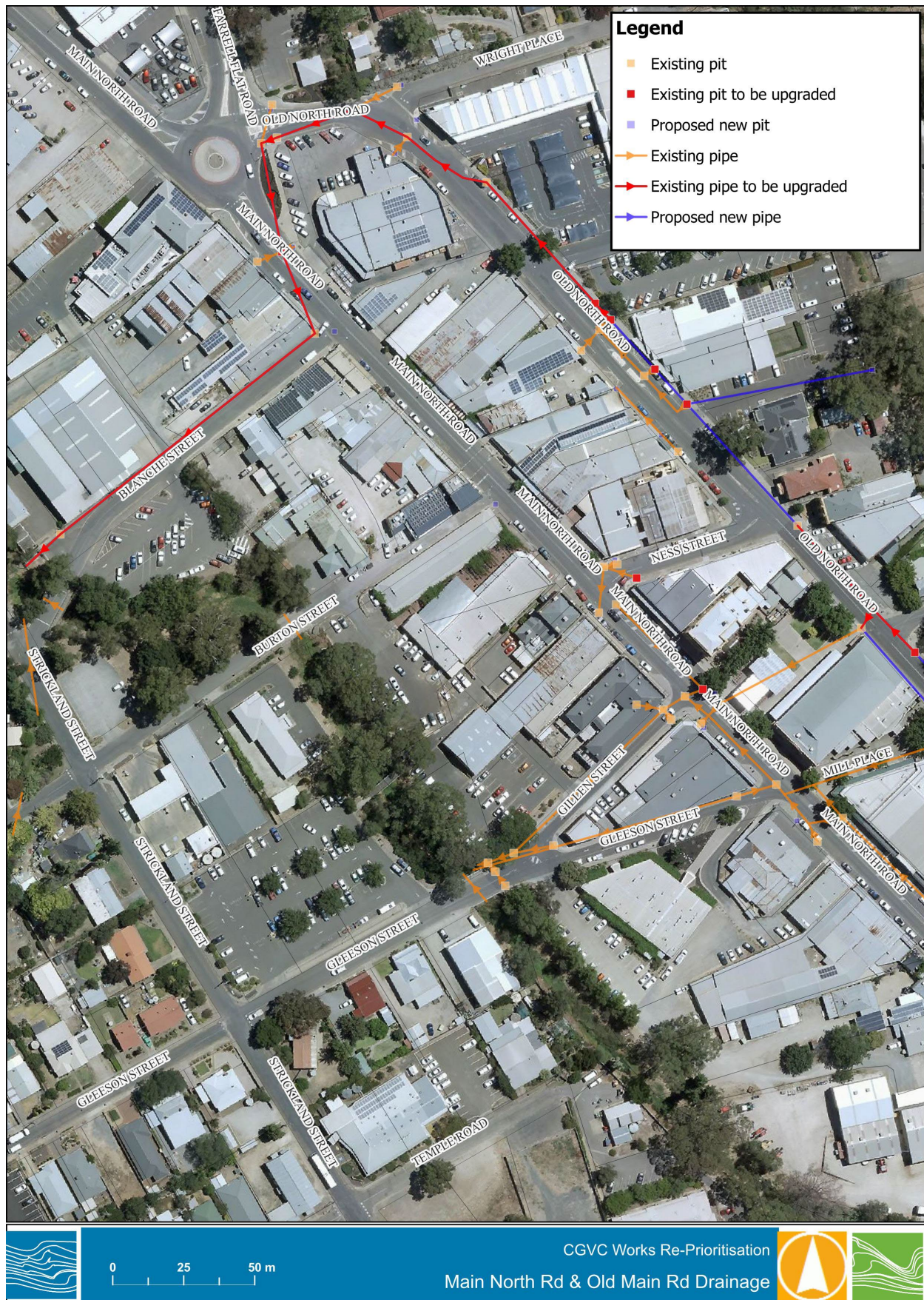
Figure 4-12 Main North Rd and Old North Rd drainage system schematisation (northern section)
